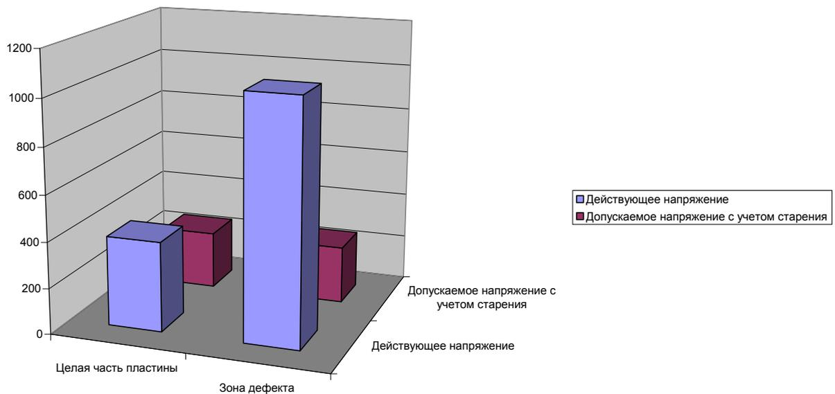
**Fig.7.** Current and the allowable stresses in the whole plate of composite and in the area of the defect considering aging according the Rules of the Russian River Register.
