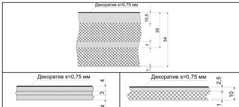
**Fig.5.** Samples of sections of the multilayer of the ship hull shell of composites
