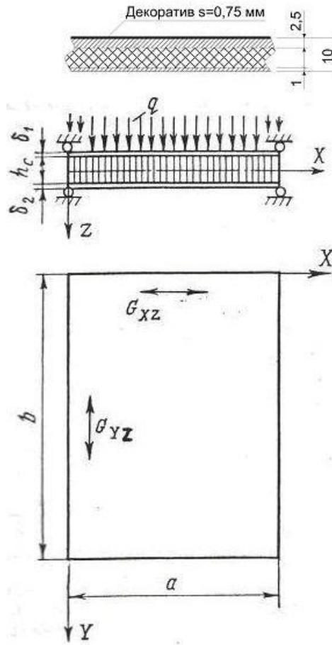
**Fig.3.** An example of a design scheme of a flat sandwich plate with light middle layer
