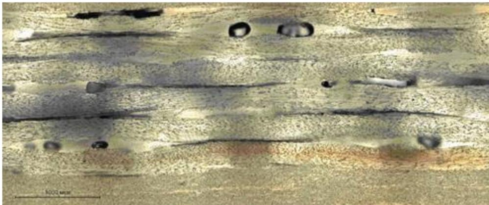
**Fig.1.** Macrograph of composite structural element, comprising delamination defects
