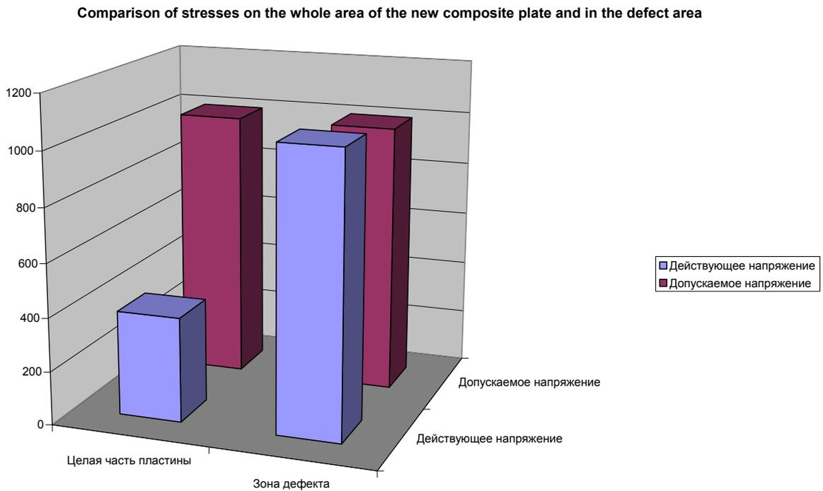
**Fig.6.** Current and the allowable stresses in the new whole plate of the composite and in the area of the defect
