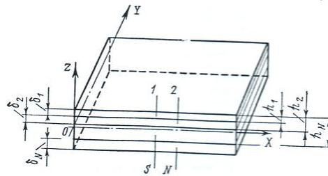
**Fig.4.** The element of the multilayer structure
